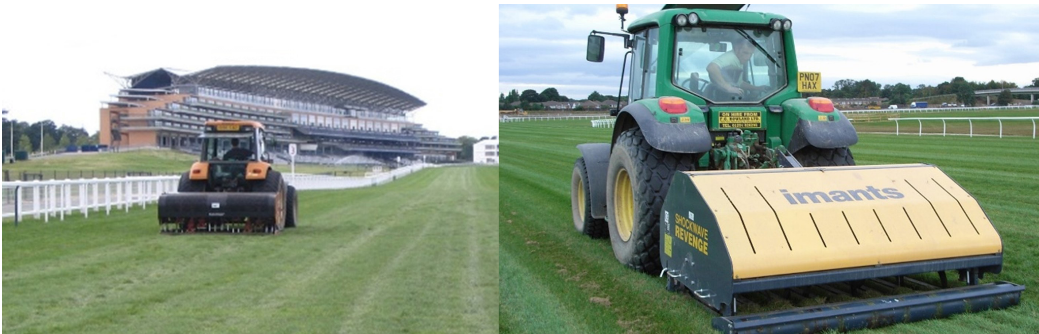
Figure 6: Examples of decompactive aerators often used on natural turf horse racetracks.
